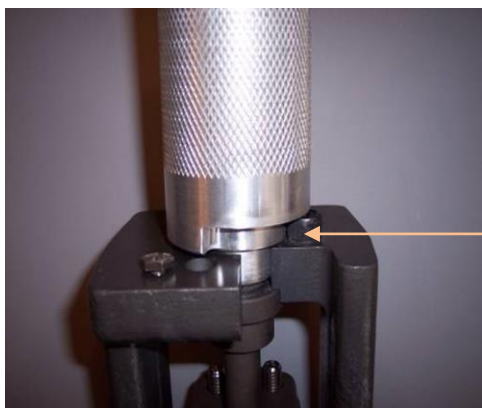
Machined Profile of the Stem Adaptor and the Mechanical Position Stop (MPS)
